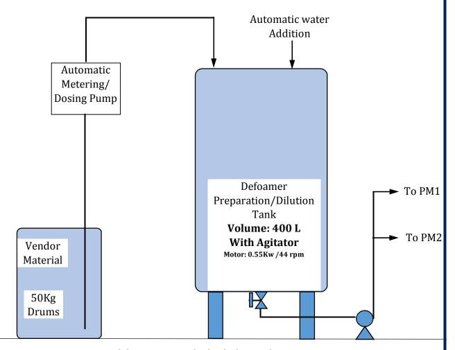
Separate delivery pumps for both the Machines.
